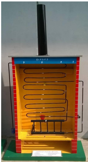
C. Benson Boiler
